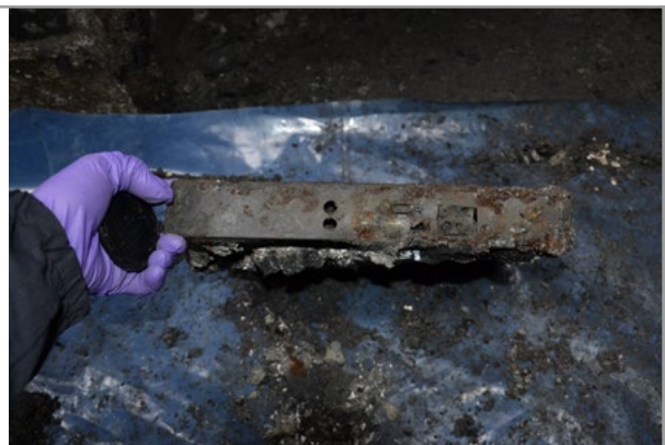
Figure 13 – Location and condition of CCTV Hard drive
