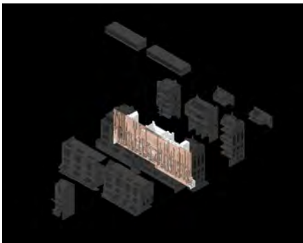
The brick spine wall defines the northern side of the circulation and houses vertical services
